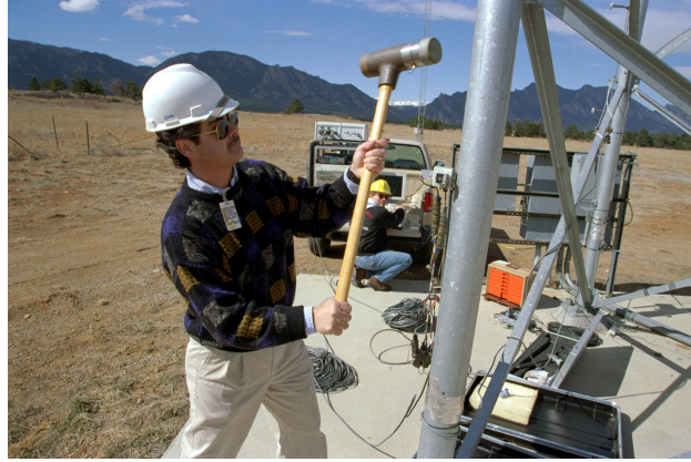
Figure 2.5: Dynamic characterization testing of a turbine in 1999. The tower is struck with a hammer and the resulting vibrations are measured with accelerometers. Photo by David Parsons, NREL 07388.
