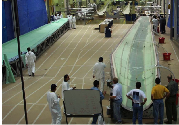
Figure 2.11: Manufacturing of a wind turbine blade. Two outer shell halves can be seen. Photo from SNL.
